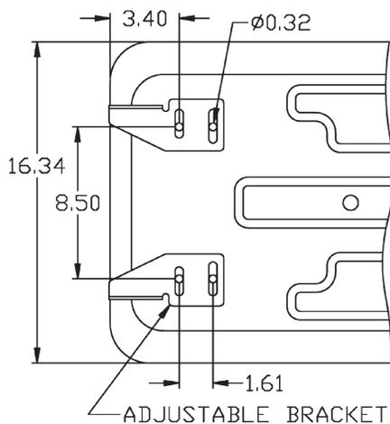
Adjustable mounting bracket for multiple uses
