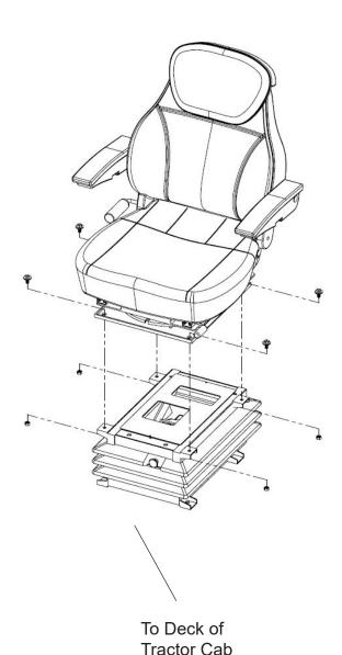
Remove the original seat and suspension assembly from the tractor.
