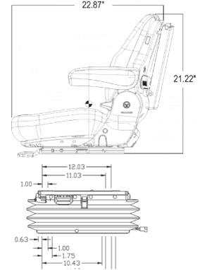
*\*Drawings show seat top without backrest extension and seat depth/tilt adjustment handles.*
