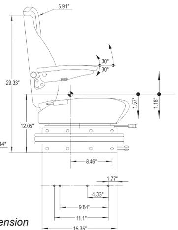
*\*Drawings show mechanical suspension only and do not show swivel.*
