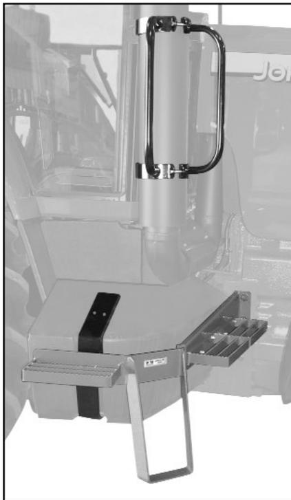
5. Fasten the lower end of the **support bracket** to the **side step section** using two 5/16" x 1" bolts and flange nuts.
