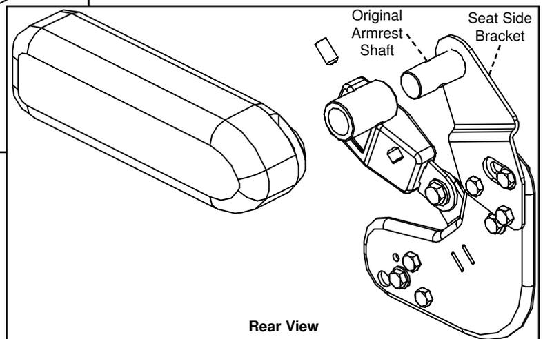
1. Remove the original armrest from the **seat side bracket** of the seat assembly.
