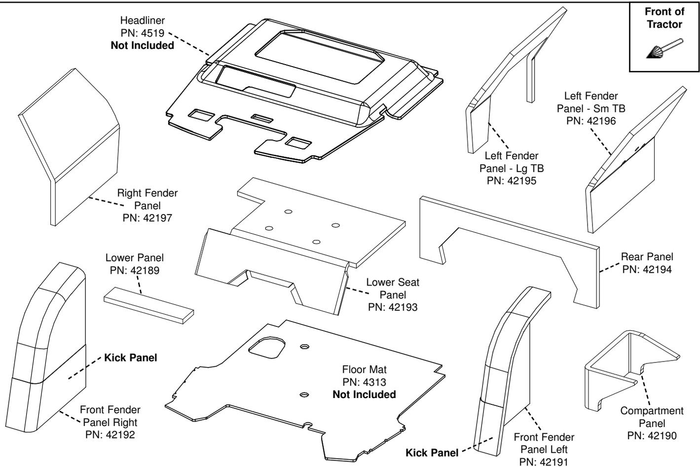
1. To make installation of your new cab foam kit easier, remove seat to allow more room to work. Also remove floor mat, ashtray, radio, AC and heater controls and vents in models where necessary.
