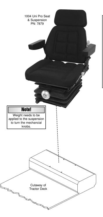
Installation Instructions to Place a 1004 Uni Pro Seat and Suspension in a Ford 7410, 7700, 7710, 7810, 7910, 8210, 8630, 8700, 8730, 8830, 9030, 9700 or TW Series Tractor
