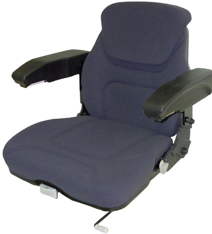
1. Pull the cushion forward as far as possible with the center lever. The seat must be in the forward most position.
