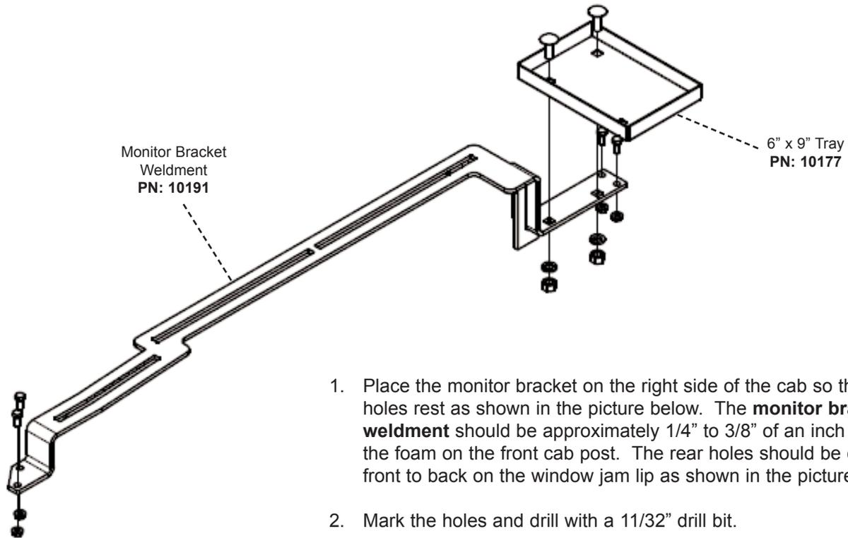
1. Place the monitor bracket on the right side of the cab so the front holes rest as shown in the picture below. The **monitor bracket weldment** should be approximately 1/4" to 3/8" of an inch away from the foam on the front cab post. The rear holes should be centered front to back on the window jam lip as shown in the picture below.
