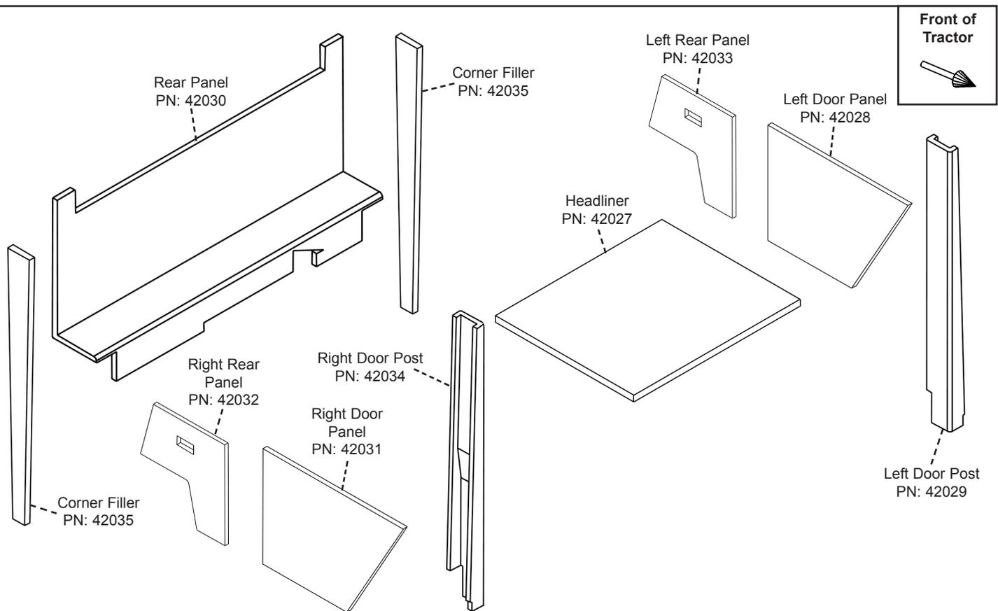
1. To make installation of your new cab foam kit easier, remove seat to allow more room to work. Also remove floor mat, ashtray, radio, AC and heater controls and vents in models where necessary.
