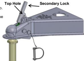
**4.** Jack up the coupler until it clears the hitch ball and pull out the Safety Clip. The coupler is now back to the unlock position, as shown in the first illustration.
