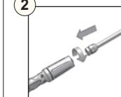
Assemble pressure washer gun to spray wand.
