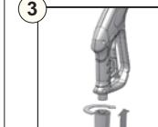
Insert high pressure hose into trigger handle.
