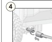
Insert high pressure hose into the pressure washer.
