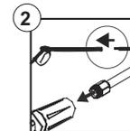
Assemble pressure washer gun to spray wand.
