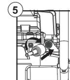
Connect the high pressure hose to the water outlet connector.
