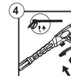
Insert high pressure hose into trigger handle.
