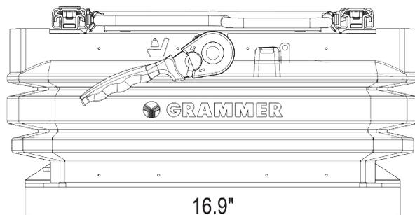
\*Front View drawing shown with handle for seat top to be installed on top of suspension in between slide rails
