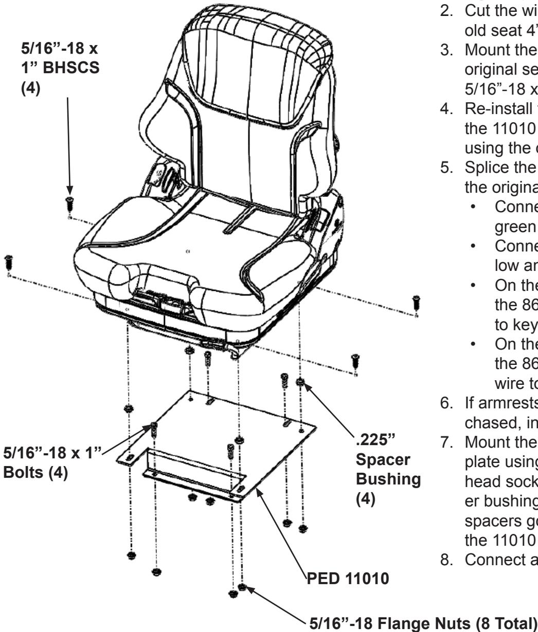
1. Remove old seat and suspension from tractor. To do so, remove the seat base plate by removing the four flange bolts and two flange nuts holding it in place.
