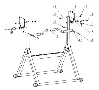
3. The two Angle Brackets each have five positive stop positions which allow the Table Top, once attached, to be positioned at five different angles. Prior to attaching the Table Top, ensure that the Brackets are set in the middle position and that the Angle Adjustment Handles are tightened securely.
