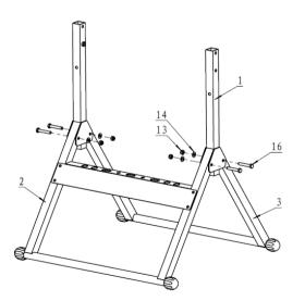
2. Attach the two Angle Brackets (4) to the Vertical Posts (1) using one Washer (14), M8 Nut (13), and Bolt M8x45 (15) per Post-Bracket assembly. Then attach the Support Brace (6) to the Vertical Posts using two Arc Washers (17), M8 Nuts (13), and M8 x 65 Bolts (18).
