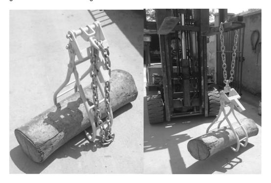
When operating, attach the tongs into the quick attach plate with a 2" receiver, change the (3pcs) tube (#3) into the tube for receiver (#12), and insert #10 into the quick attach hitch receiver plate. The 2 inch receiver fits into the quick attach hitch receiver plate on a tractor or a skid steer with the L Pin (#9).
