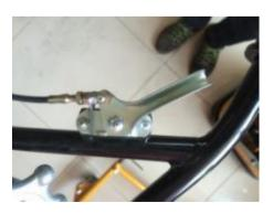
8. Check that the engine throttle lever (silver lever in picture) is at its idle position (fully left in picture) then attach the Accelerator Cable position (3) and wire (4).
