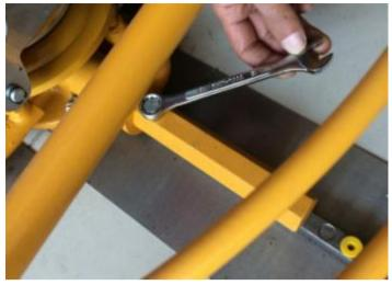
4. Loosen the outside bolt with the 1/2 in. wrench (Fig. 3).
