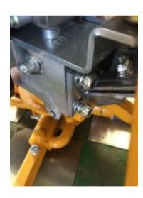
3. Turn the Blade Pitch Handle counter-clockwise.
