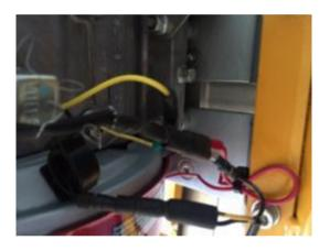
12. Remove a bolt from the engine housing, put the ring terminal of the Engine Stop Switch over the bolt, replace the bolt and retighten it.
