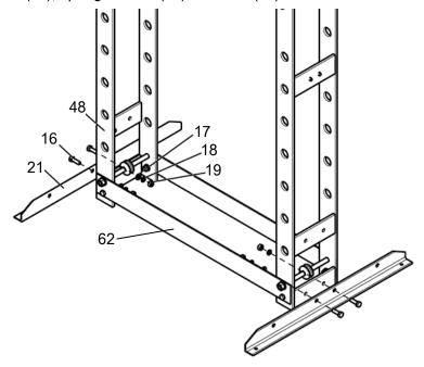
2. Attach side support rails (20) to base support sections (21) and frame (48) with bolt (16), washer (17), spring washer (18) and nuts (19).
