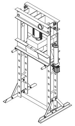
4. Close the release valve by turning it clockwise until it is firmly closed.
