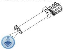
5. Fill the oil case until oil level is just beneath the lower rim.
