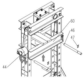
2. Place bolster plates on press bed frame (59).
