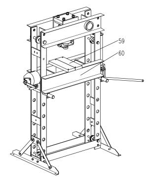
3. Place work piece on the bed frame or pressing block, use every precaution necessary to ensure safety and to prevent accidents. Position work piece in a manner which will not allow it to inadvertently fall from the bed frame or pressing block.
