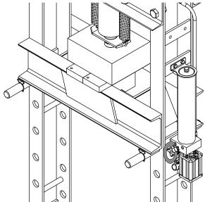
5. Connect the air hose inlet fitting onto the shop air supply hose lock fitting, pump air into the system until the ram nears the work piece. Then release the trigger when pumping needs to stop. **OR** When an air source is unavailable, pump the handle until the ram nears the work piece.
