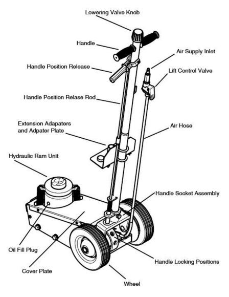
2. Refer to picture when performing this step. Take off the screw located on handle piece 1; Attach handle pieces 1 and 2 making sure to align the holes on both sections. Reinsert the screw and tighten. Check to that handle is in perfect alignment with internal lowering valve mechanism. (Handle lowering mechanism must be in perfect alignment or release mechanism will not work.).
