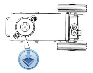
6. Fill the oil case until oil level is just beneath the lower rim of the oil fill hole.
