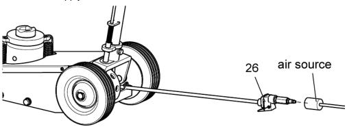
3. Close the release valve by turning the handle knob clockwise until firm resistance is felt.
