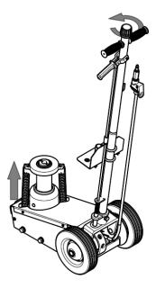
5. When the saddle reaches Min. Lift Height, with a flat blade screwdriver, push the oil fill plug slightly to the side to purge trapped air from system.
