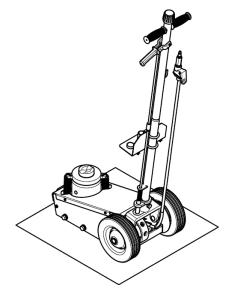
2. Open release valve by turning handle counterclockwise.
