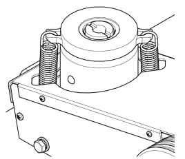
6. After removing jack from under the load, push ram and handle sleeve down to reduce exposure to rust and contamination.
