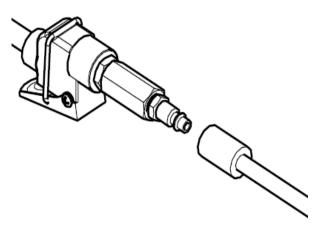
6. Inspect before each use. Do not use if bent, broken or cracked components are noted.
