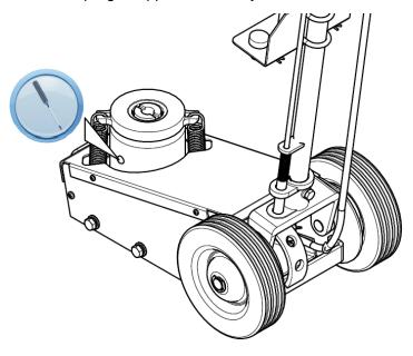
6. Close the release valve by turning the handle knob clockwise until firm resistance is felt.
