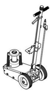
11. After lifting, support the load with appropriately rated vehicle support stands before working on the vehicle.
