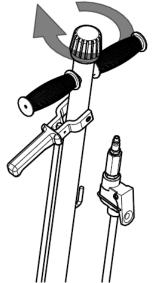
4. When the saddle reaches Max. Lift Height, turn the handle knob counter-clockwise.
