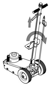
7. Connect air source to the air supply inlet (26).
