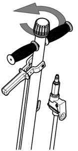
5. After removing jack from under the vehicle, fully retract the jack to reduce ram exposure to rust and contamination.
