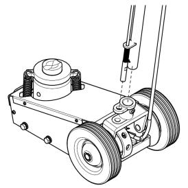
5. Turn the jack on its side so that old oil will drain from the oil fill hole.
