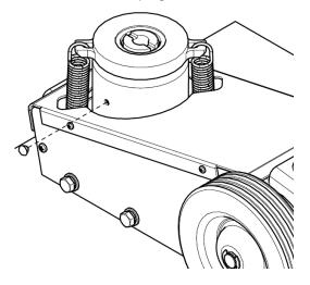
3. Fill the oil case until oil level is just beneath the lower rim of the oil fill hole.
