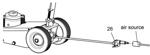
8. Close the release valve by turning the handle knob clockwise until firm resistance is felt.
