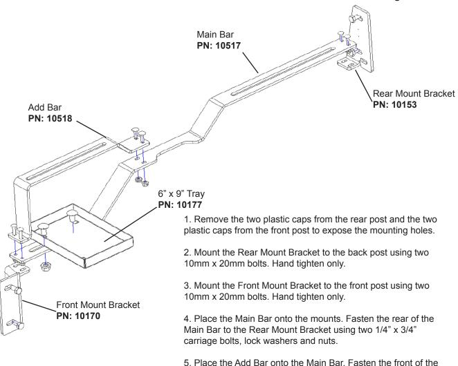
6. Fasten the back of the Add Bar to the Main Bar using two 1/4" x 3/4" carriage bolts, lock washers and nuts.
