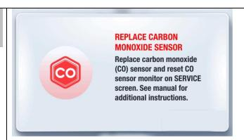
The carbon monoxide sensor has reached the end of its life. The generator will not operate when the CO sensor reached the end of its life. To ensure proper operation of the generator, replace the CO sensor prior to its expiration.
