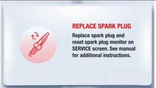
The spark plug has reached the end of its life. To ensure proper operation of the engine and generator, replace the spark plug. Refer to engine owner's manual for instructions. After completion, reset the spark plug monitor on the service screen.
