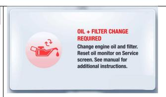
An oil change and oil filter change are required for proper maintenance of the engine. Refer to the engine owner's manual for instructions.
