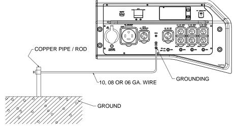
If a licensed electrician installs the generator with a connection to your building's electrical circuit for use as a back-up power system, grounding may alternatively be completed through the building's grounding system. Ask your electrician. If the generator is not grounded through your building's electrical system, follow the procedure above.
