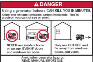
The Carbon monoxide control system will flash the above "**carbon monoxide poisoning**" notification on the LCD Display and shuts down the generator when the carbon monoxide is at dangerously high levels.
