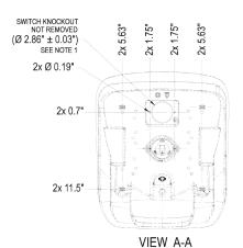
NOTES: 1) SEAT SHELL INCLUDES A SECOND SWITCH MOUNT LOCATION WITH A PLUG THAT MAY BE REMOVED BY THE CUSTOMER. SEAT HAS BEEN QUALIFIED WITH SWITCH 20178 IN BOTH POSITIONS. IF TWO SWITCHES ARE INSTALLED, THEY ARE TO BE WIRED IN PARALLEL, NOT IN SERIES.
