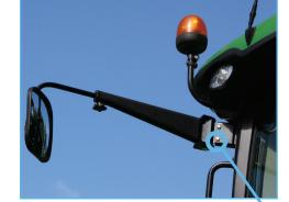
Length easily adjustable from 22" - 36" to allow sight around any implement or trailer
