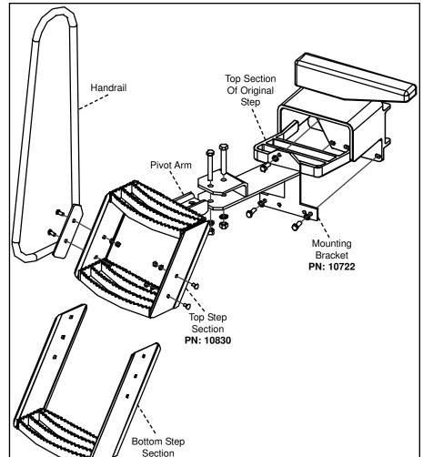
of the **top step section**. Adjust to the desired height and fasten with two 3/8" x 3/4" carriage bolts and flange nuts in the rear holes.
