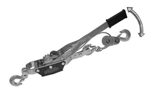
3. **Pull Load.** Keep moving the lever handle back and forth until the load is pulled to the desired position.
