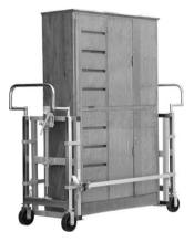
The cabinet being transported must not be left unattended on the equipment; it must always be lowered onto the floor.
