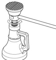
5. Rotate steel handle bar counter-clockwise to raise the lifting support until the desired height is reached.
