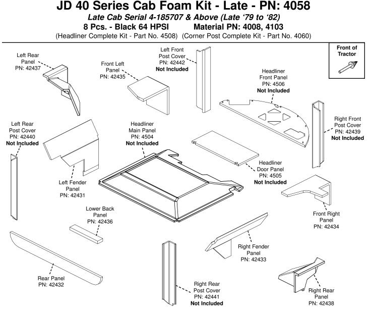
1. To make installation of your new cab foam kit easier, remove seat to allow more room to work. Also remove floor mat, ashtray, radio, AC and heater controls and vents in models where necessary.
