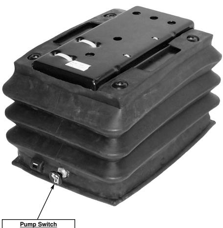
Push switch to activate pump. Pull to release air. Note: Weight must be applied to the suspension to activate the pump.
